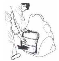
**2.** Lift and slide out galvanized steel liner using the two drop handles.
