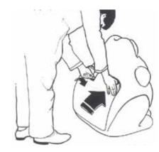
**5.** Simply push door panel back into its original position and lock with special key provided.
